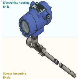
The Electronics Housing has two sides (compartments): terminal enclosure side/compartment and the electronics side/compartment. The two sides/compartments are separated by a potted bushing.
