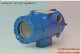
The electronics side/compartment uses Type of Protection Ex ia even though the Electronics Housing is an Ex db enclosure. The other side, terminal enclosure side/compartment, also uses Type of Protection Ex ia even though the Terminal Housing is an Ex db enclosure. This use of Ex ia is to permit removal of the covers from the electronics side/compartment and/or the terminal enclosure side/compartment while circuits are energized.
