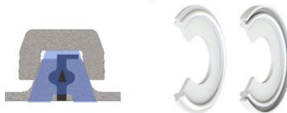
Figure 4: Block "A" Profile / Standard & Flanged Gaskets
