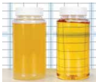
Contaminated Fuel - emulsified water with free water at bottom
