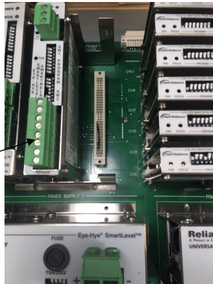
FIGURE 2 – SmartRelay installed in Motherboard
