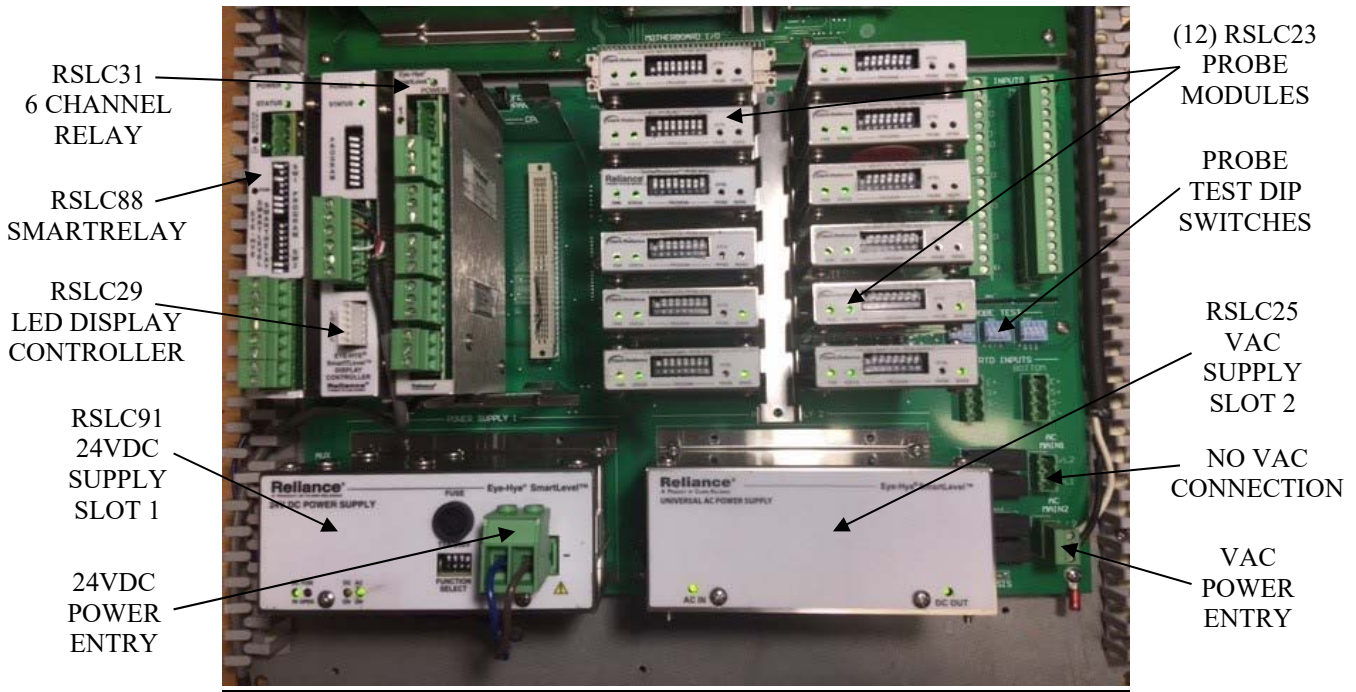
FIGURE 16 – Typical REESC-12 SmartLevel System with the RSL88 Smart Relay and the AC/DC power supply options installed.
