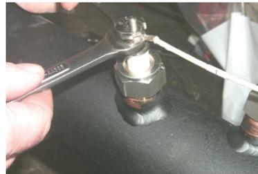
The high temperature wires attached to the probes can be routed to a local junction box or directly to the control unit. If a junction box is used, a low cost 18 Ga. Multi-conductor cable may be used to carry the signal to the control unit. We suggest Belden #8467 or equal.
