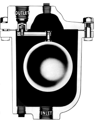
Body is high pressure cast iron (ASTM Class 30) for pressures to 250 PSIG @ 450° F. or 300 PSIG @ 150° F. All internal working parts are stainless steel including discs, seats and floats. Valve points are guided to assure positive closing.
