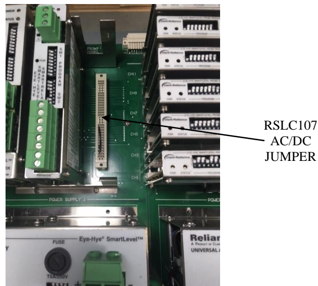
FIGURE 6 – Both 24VDC RSLC91 & AC RSC25 Installed
