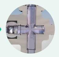
Then open the bottom valve to the bypass position. Fluid will now flow through the valve and into the glass without seating the ballcheck.
