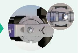
Once the level stops rising, move both valves to the run position. Now, the valves are ready for normal operation. If your level gage is not maintained properly or a leak occurs, the ballcheck will engage and isolate the gage from the vessel.
