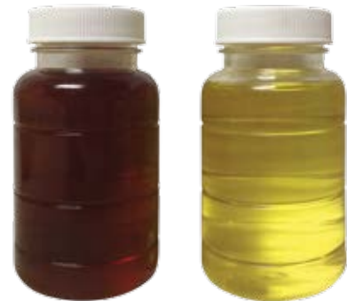
Before Filtration ISO 22/21/19 MPC* Value = 38
