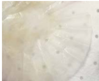
Cooler Bundle Flush – Final Inspection Screen (After Flush)
