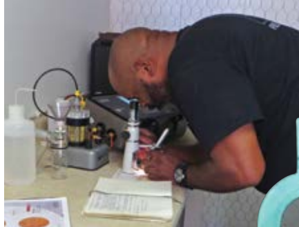
On site oil analysis at a power plant in Mexico
