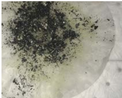
Cooler Bundle Flush – Initial Inspection Screen (Before Flush)
