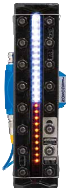
Transparent gage with illuminator showing 45% oil
