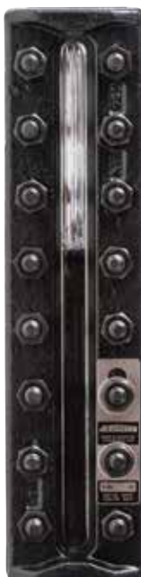
Reflex level gage showing about 60% oil
