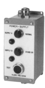
Any Clark-Reliance Relay Control Unit can be wired to operate from two power sources. Operation can switch automatically between power sources A and B in the event of an outage. Each power source is fused at 5 AMPS. Each fuse is accessed from front of the unit. A push button permits the momentary testing of the standby power source. Visual illumination provides indication of the power source in use. Dimensions: 8" x  $3^{1/4}$ " x  $2^{3/4}$ "
