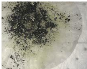
Initial Inspection Screen (Before Flush)
