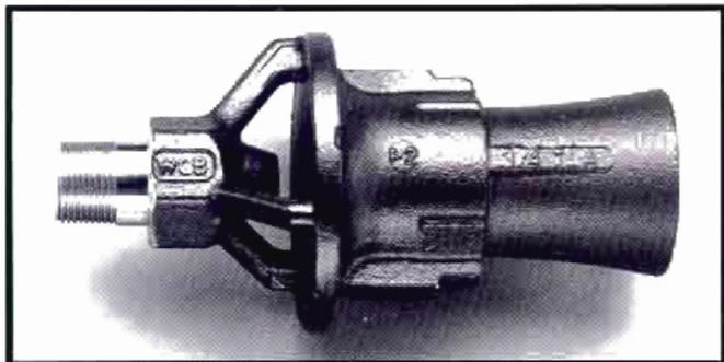
**The Jacoby-Tarbox® Tank Liquid Agitator (JT TLA)** is an eductor designed for "in-tank" applications. The TLA operates on the principle of flow dynamics. Pressurized fluid is accelerated through the nozzle to become a high velocity stream that entrains tank contents and intimately mixes with them. This combined stream exits the TLA at a high velocity creating a flow field capable of causing additional agitation and mixing the tank contents.
